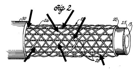
As can be clearly seen, the longitudinal warp members 28 are clearly not disposed <u>between</u> the helical members 24 for <u>the entire length</u> of the longitudinal warp member 28.
